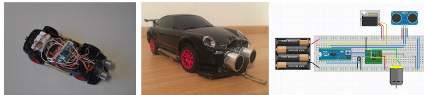
Fig. 9. Prototype of the model car and circuit diagram
