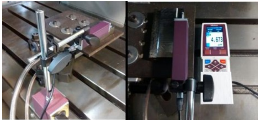
Fig. 4. Roughness method of analysis used after experiments
