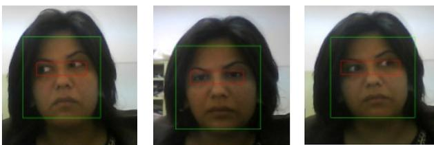
Figure 2. Detection results of both face detection and eye localization
