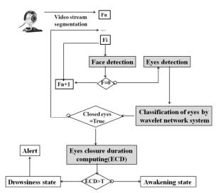
Figure 1. Complete framework of drowsiness detection system
