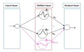
Figure 4. A wavelet network architecture based on the FWT
