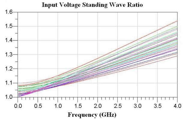
Figure 9. Input Voltage Standing Wave Ratio
