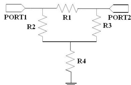
Figure 4. The equivalent circuit of Bridged-Tee attenuator
