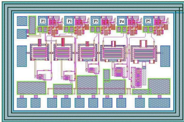
Figure 6. The layout of Wideband 5-bit MMIC digital attenuator with high precision
