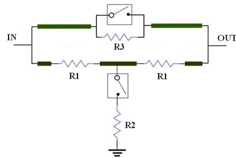
Figure 2. Bridged-Tee attenuator
