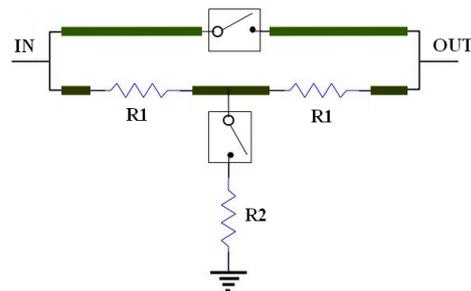
Figure 1. Tee attenuator
