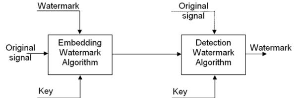
Figure 10. Basic watermarking system
