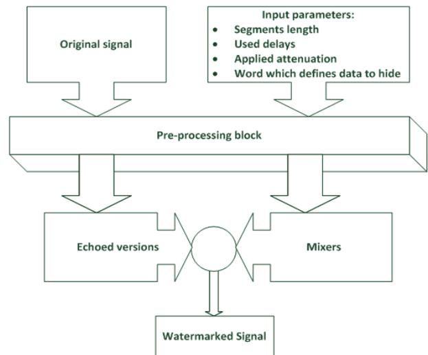
Figure 11. Embedding process scheme
