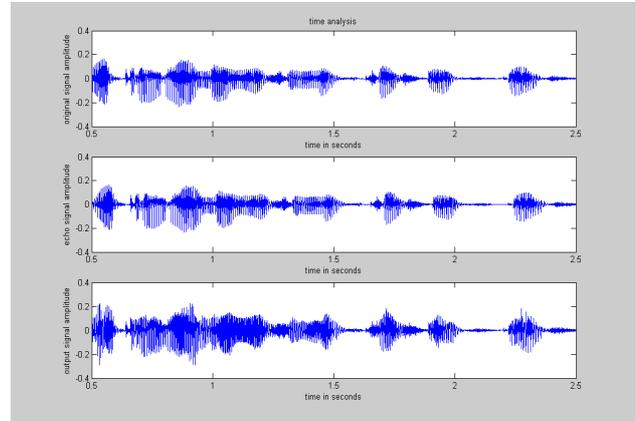
Figure 14. Time analysis of the original signal, its echo, and the output signal (the watermarked signal)
