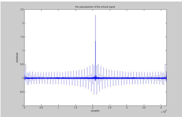
Figure 9. The autocepstrum of the echoed signal
