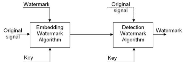
Figure 10. Basic watermarking system
