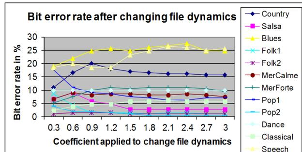
Figure 19. Error rate in watermarks detection after changing dynamics tests
