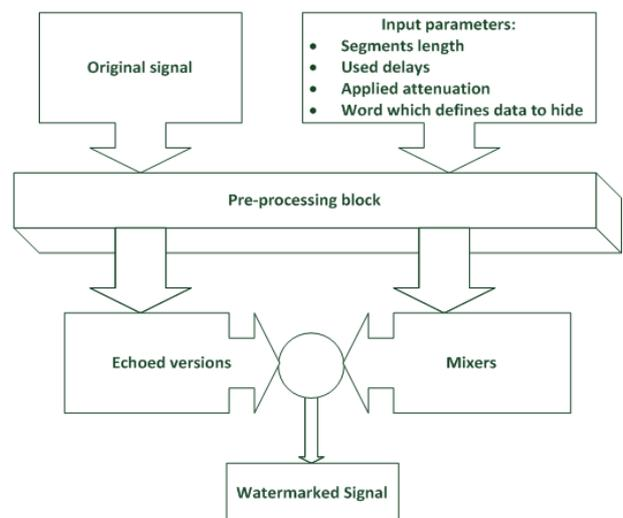
Figure 11. Embedding process scheme
