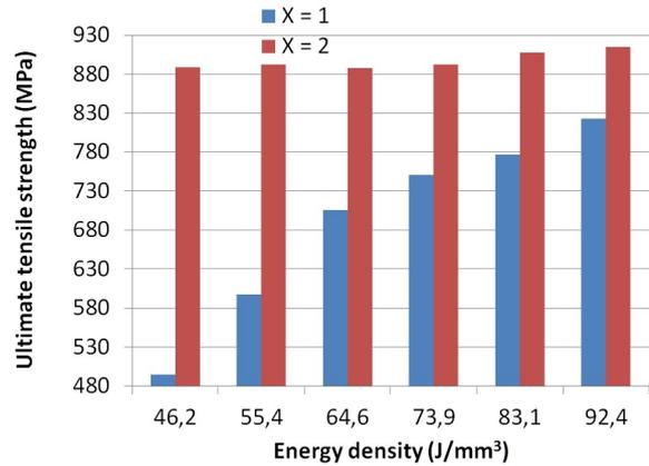
Figure 5. The mean values of the ultimate strength (Rm) obtained for all of the sample variants.
