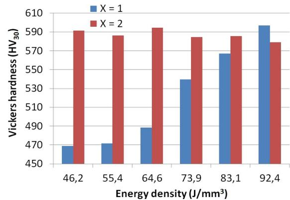
Figure 6. The mean values of the Vickers hardness (HV<sub>30</sub>) obtained for all of the sample variants.
