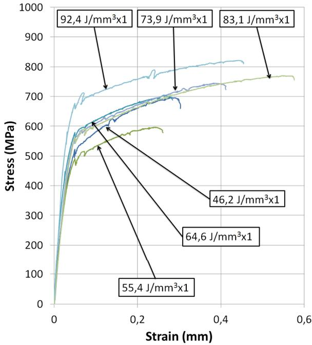
Figure 3. Tensile curve diagrams obtained for the samples on which one laser beam pass over each patch was used.
