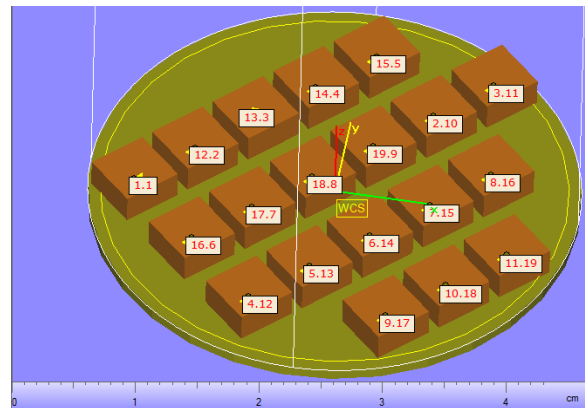
Figure 5. Arrangement of 5 mm-cuboid samples on the build platform
