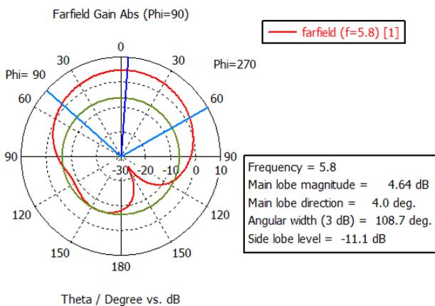
Figure 17. Far field in polar view for Bakelite.
