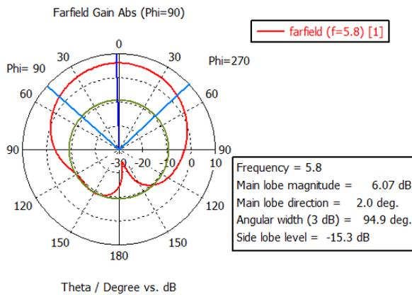
Figure 11. Far field in polar view for Arlon Di 522.
