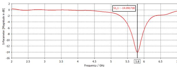
Figure 15. Return loss for Bakelite.
