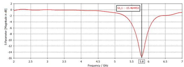
Figure 12. Return loss for Taconic RF 35P.
