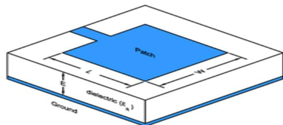
Figure 1. Structure of Patch antenna [3].
