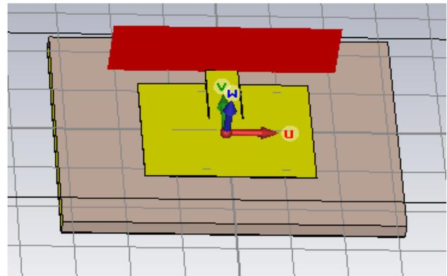
Figure 2. Designed Microstrip Patch Antenna for 5.8 GHz.
