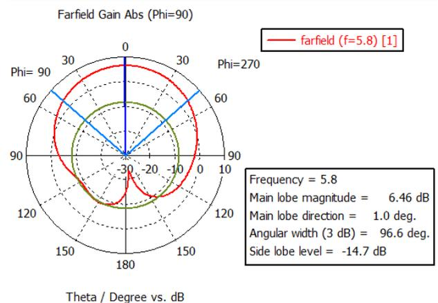
Figure 8. Far field in polar view for RTDuroid 5880.
