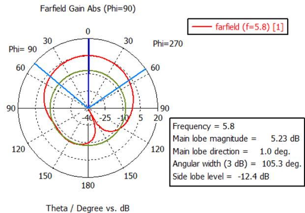
Figure 14. Far field in polar view for Taconic RF 35P.
