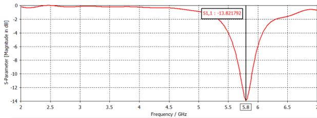
Figure 9. Return loss for Arlon Di 522.
