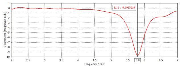
Figure 6. Return loss for RTDuroid 5880.
