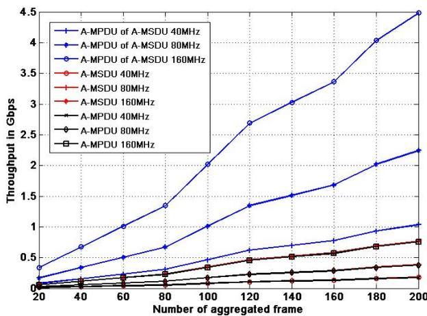
Figure 7. Throughput for the RTS/CTS access scheme
