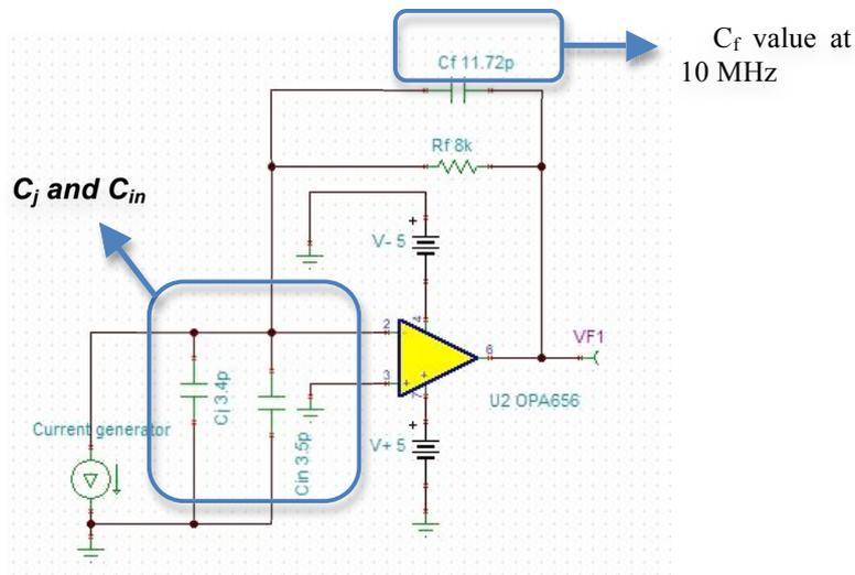
Fig. 2. TIA circuit in TINA<sup>TM</sup>-SPICE<sup>®</sup> in OPA656 simulation case
