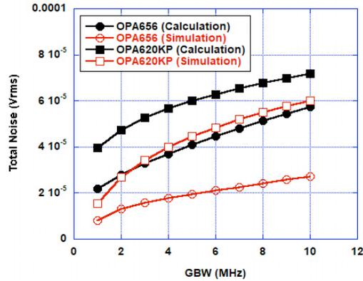
Fig. 4. Comparison results using mathematical calculation and simulation approach to investigate the GBW against NTot of the two Op-Amps
