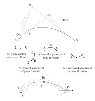
Fig. 3. Diagram of virtual design of curving wall
