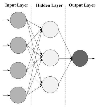
Fig. 3. Basic structure of a neural network
