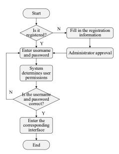
Fig. 4. System login process
