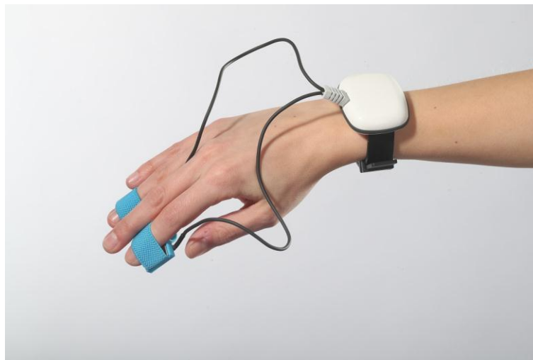
Fig. 1. Position of GSR sensors Sensetio on respondent's hand
