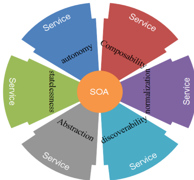
Fig. 4. The principles of service-oriented architecture
