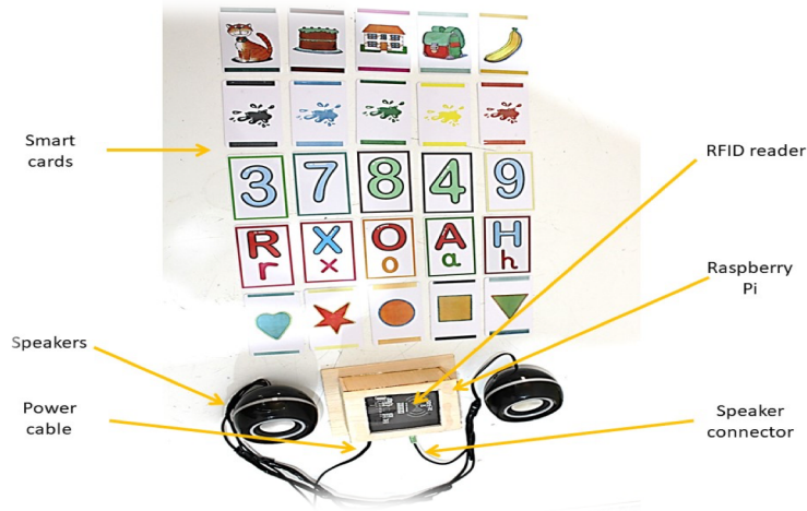
Fig. 1. The structure of the developed educational toy
