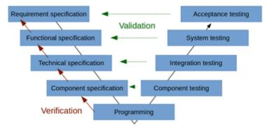
Fig. 1. General V-model (based on [3], p.42)
