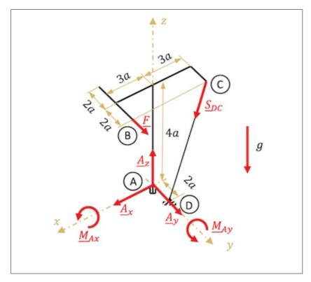
Fig. 5. Free-body diagram of the example problem described in chapter 3.3.
