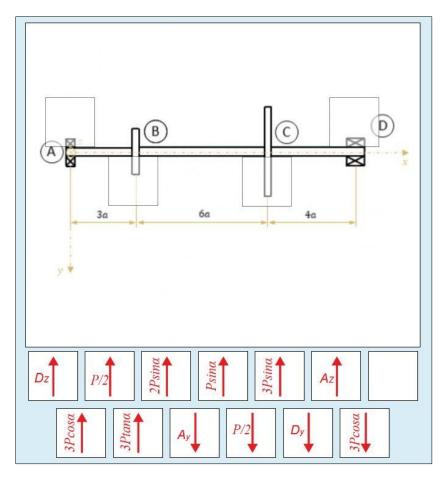
Fig. 2. Free-body-diagrams can be realized with Drag-and-Drop question types in Moodle
