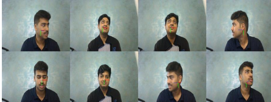
Fig. 2. Head pose angles depicted by the blue (yaw), red (pitch), and green (roll) lines.
