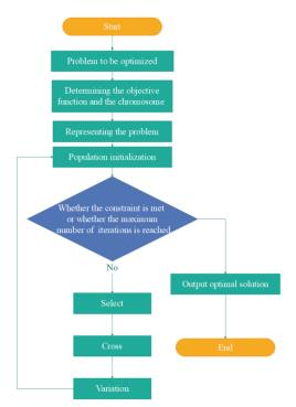
Fig. 1. Operational flow chart of genetic algorithm
