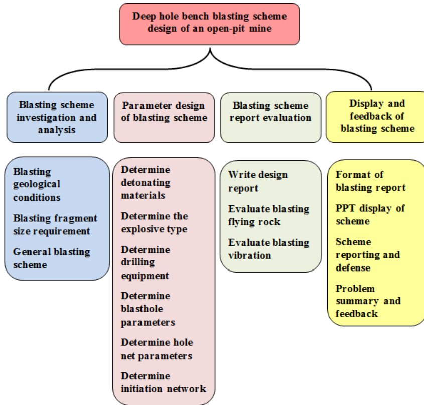
Fig. 3. Content and task decomposition of the deep hole bench blasting project of an open-pit mine
