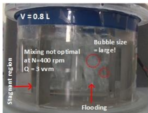
Fig. 4. Results of the image analysis about mixing events in a lab scale bioreactor. The image was produced by one of the group using the Kinovea and Microsoft Visio software.
