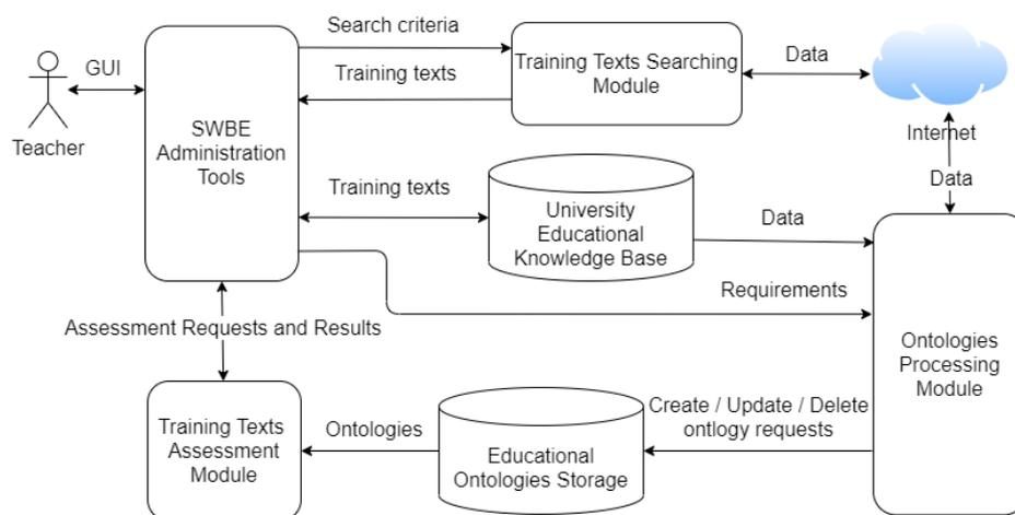
**Fig. 1.** Component scheme of an information system intended for automated web search and analysis of training texts
