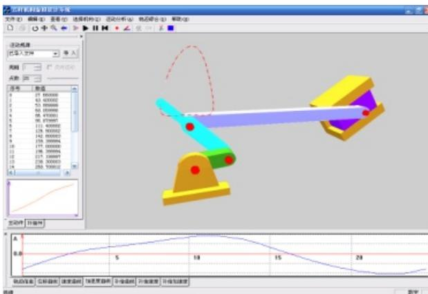
b) Virtual design system of the controlled five bar mechanism
