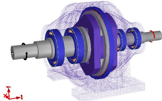
Figure 10. The virtual prototype model of NGW31 planetary gear reducer
