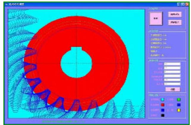
d) Gear forming simulation software
