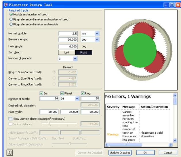
Figure 8. The conceptual model in planetary gear
