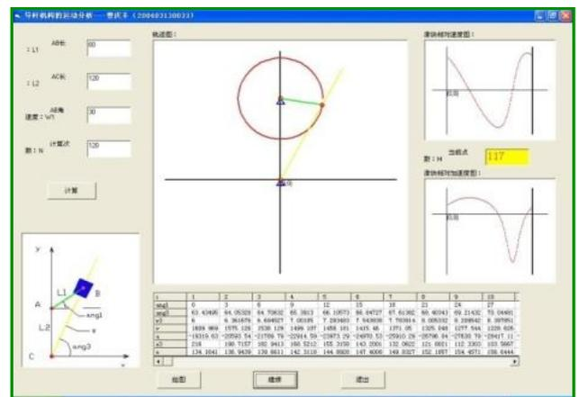
f) Simulation software guide bar mechanism
