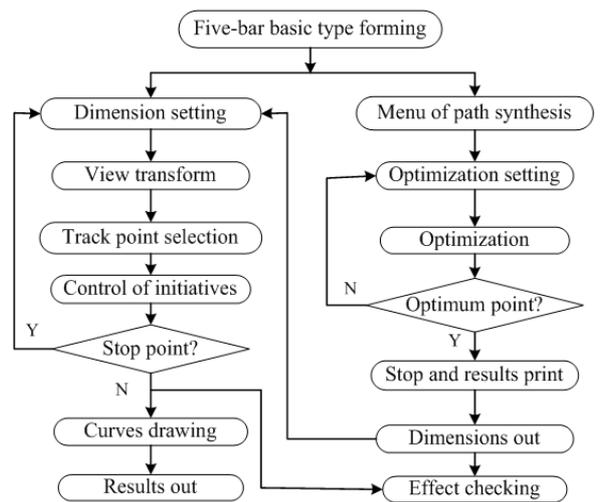
Figure 5. Operating sequence of two main functions
