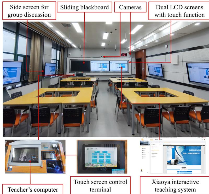
Fig. 4. The MSILS installation in the smart classroom
