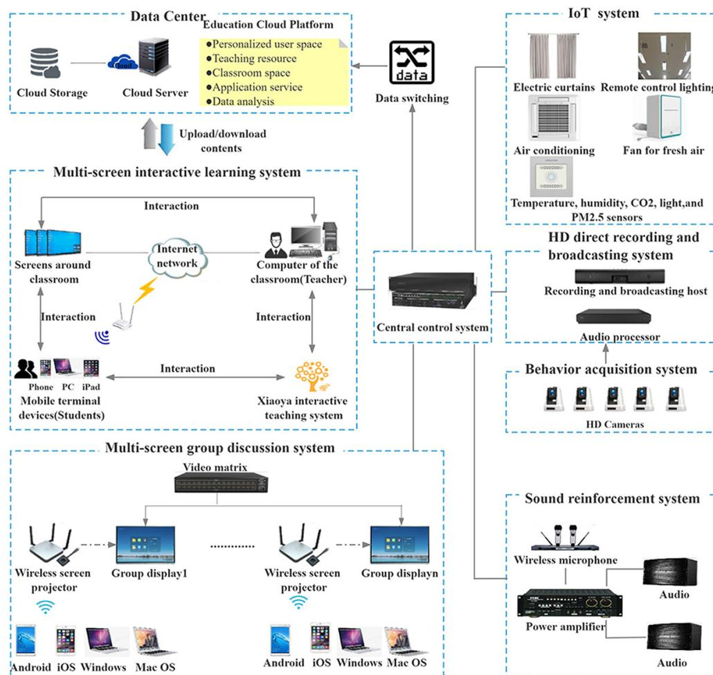
Fig. 1. Smart classroom architecture based on the MSILS
