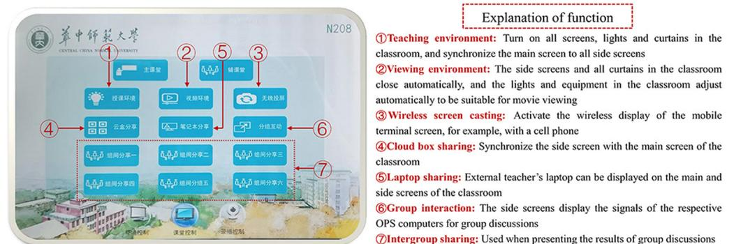
Fig. 5. Function diagram of touch screen control terminal
