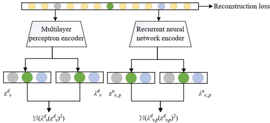
Fig. 2. Encoder structure
