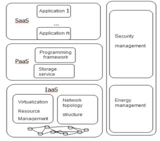
Figure 1. Three layer service model of cloud computing
