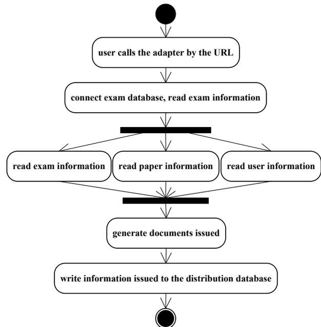
Figure 4. The program flowchart of adapter
