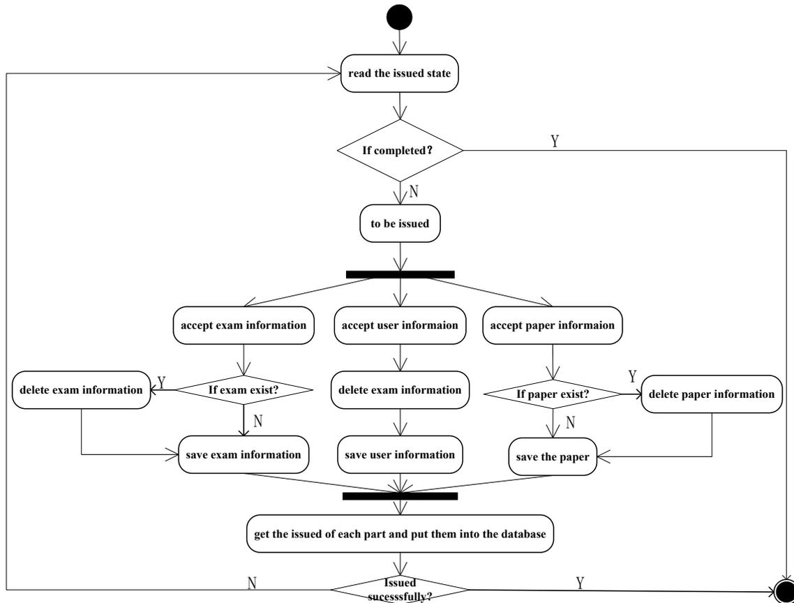
Figure 5. The program flowchart of data distribution
