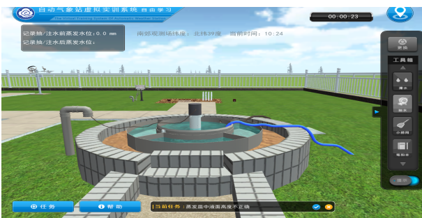
Figure 5. (d) Adjusting liquid height of evaporating dish
