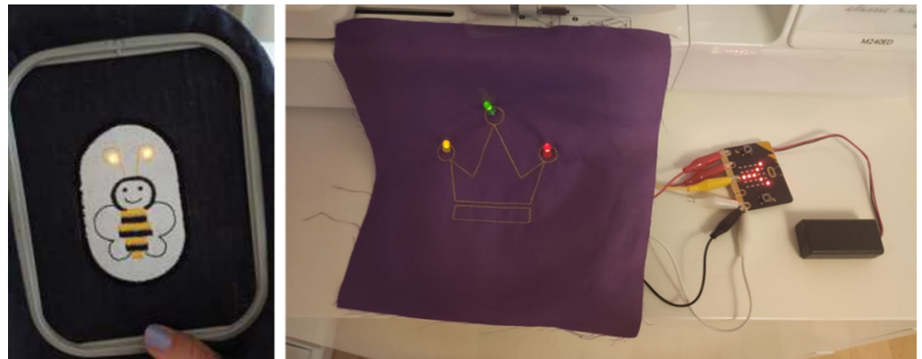
Fig. 14. Connection of embroidery designs and e-textiles or to "smart wearables"
