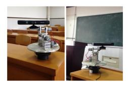
Fig. 4. A Kinect is installed upon the 3-axis motion platform
