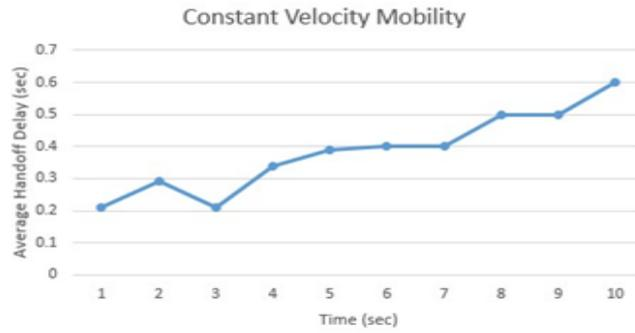
Fig. 5. Average Handoff delay against Time for Constant Velocity in NDN
