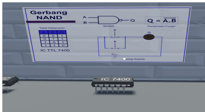
Fig. 11. IC Gate Characteristic Command
