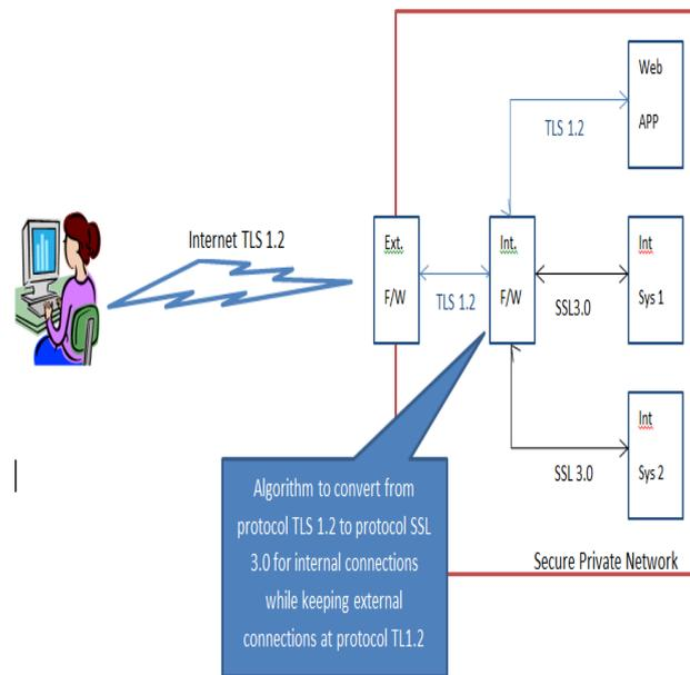
The solution shown in the picture above corresponds to the secure protocol version downgrade as implemented using the solution explained in the previous sections of this document.
