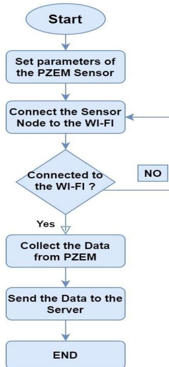
Fig. 8. IoT-based Modbus EMS flow chart
