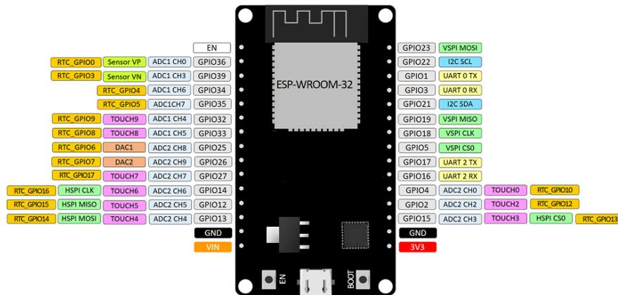
Fig. 5. The ESP32 microcontroller
