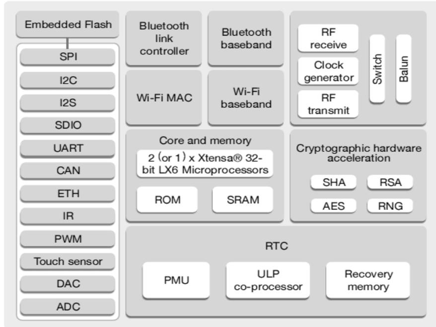
Fig. 6. The block diagram of the ESP32
