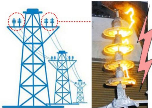
**Fig. 1.** Transmission line and flashover on an insulator [5]
