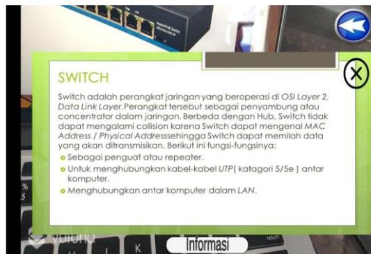
Fig. 17. Information of Switch Device
