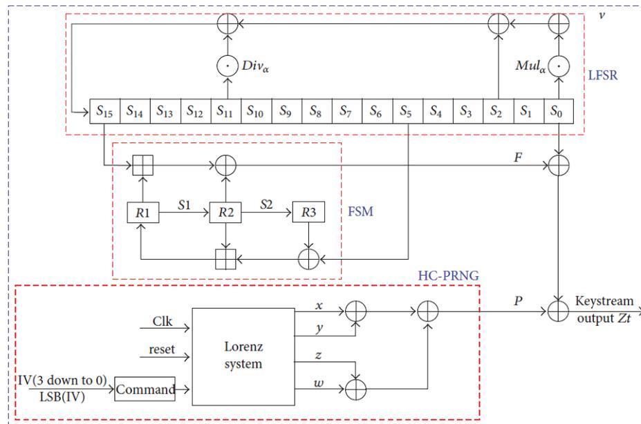
Fig. 4. The keystream architecture of our hyperchaotic SNOW-3G cipher stream method [25]
