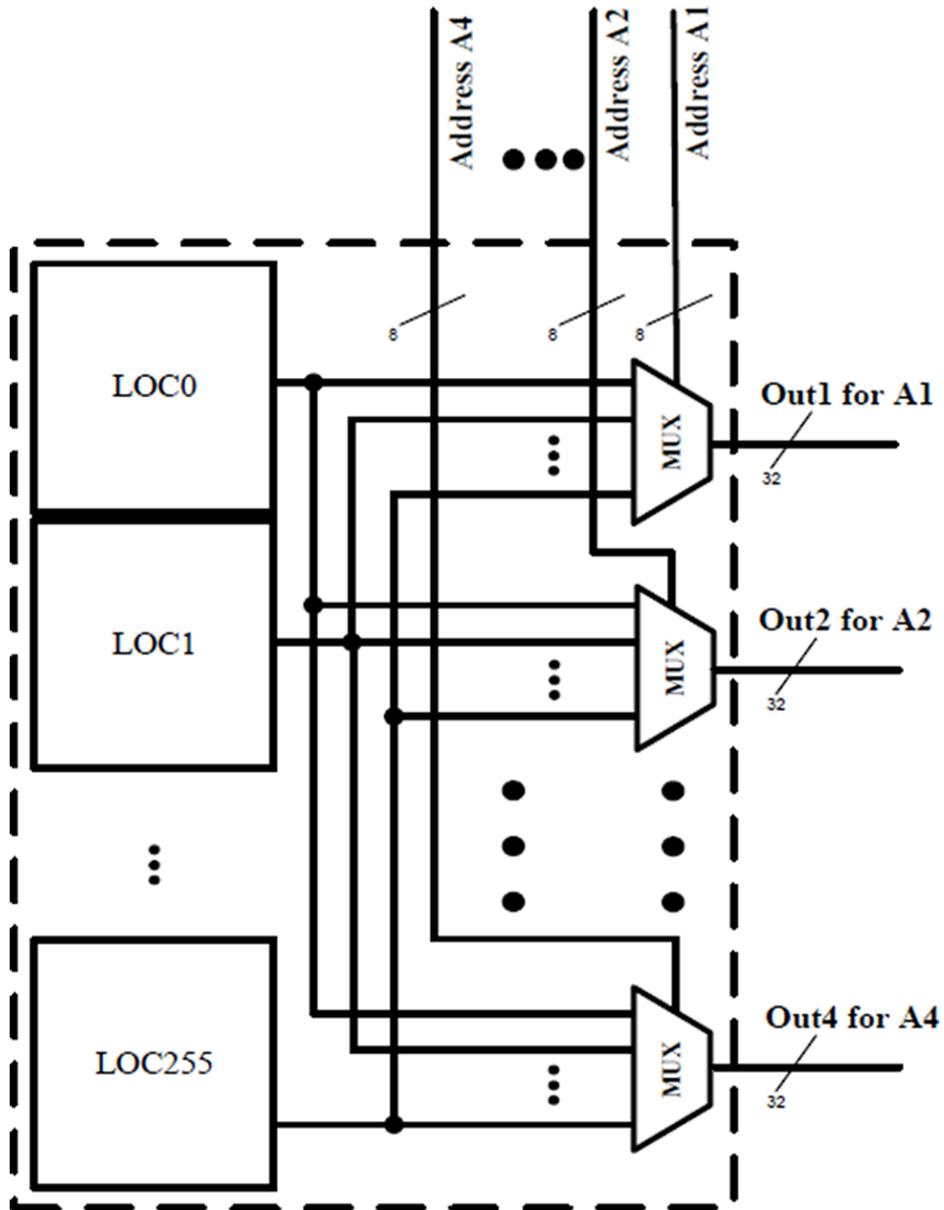
Fig. 6. New S-Box architecture 2 [30]
