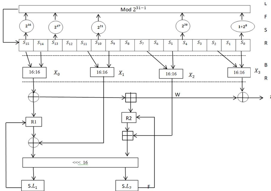
Fig. 8. Architecture by ZUC algorithm [34]
