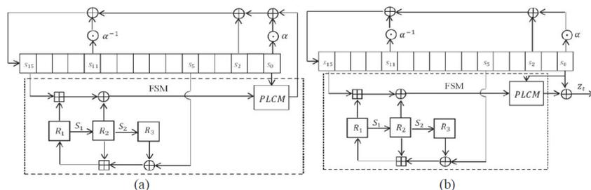
**Fig. 3.** (a) Modified key initialization method in SNOW 3G
