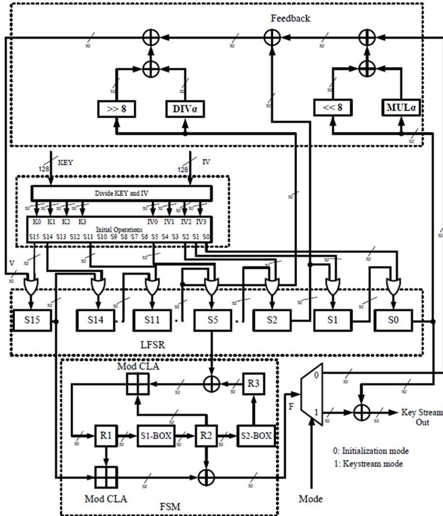
Fig. 7. Optimized SNOW 3G architecture of Internal block diagram [30]
