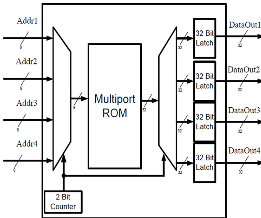
Fig. 5. New S-Box architecture1 [30]
