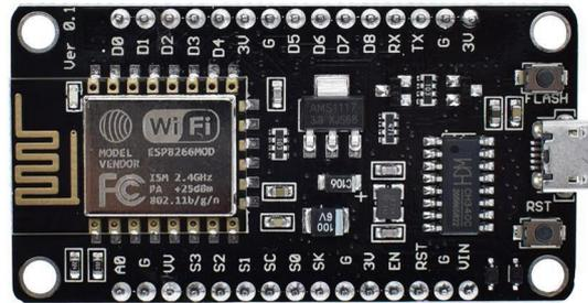
Fig. 1. NodeMCU v3 board structure
