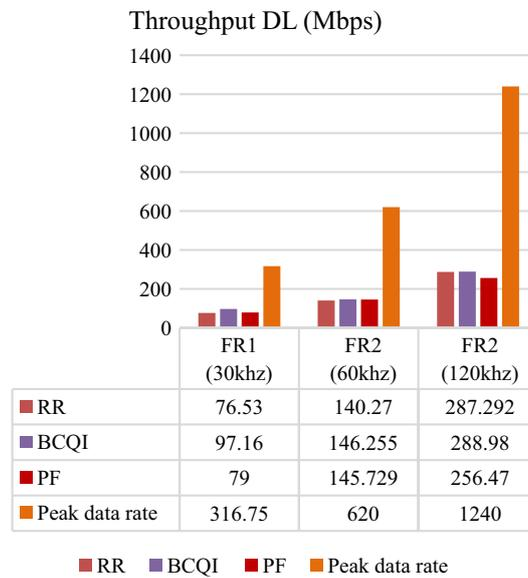
**Fig. 3.** Downlink throughput for VoIP traffic
