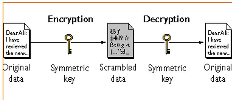
Fig. 1. Symmetric key cryptography
