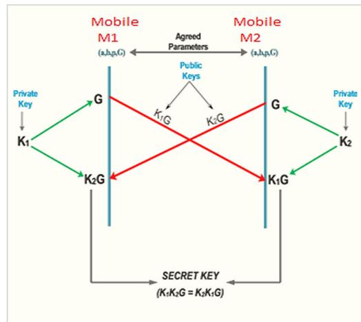
Fig. 6. Elliptic curve Diffie-Hellman exchange
