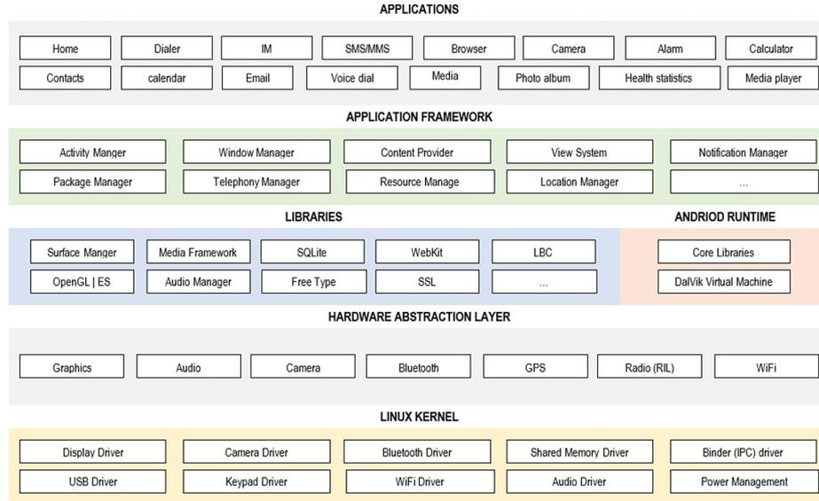
Fig. 3. Architecture of Android OS
