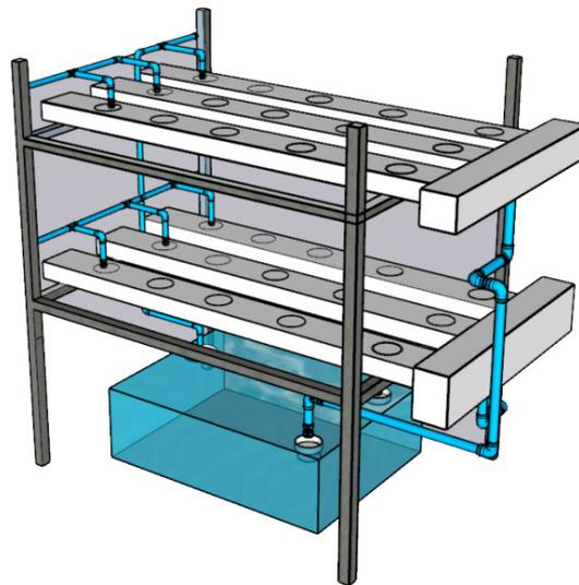
**Fig. 1.** Prototype design of NFT hydroponics system
