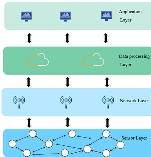
Fig. 3. Four-layer architecture of a sensor network
