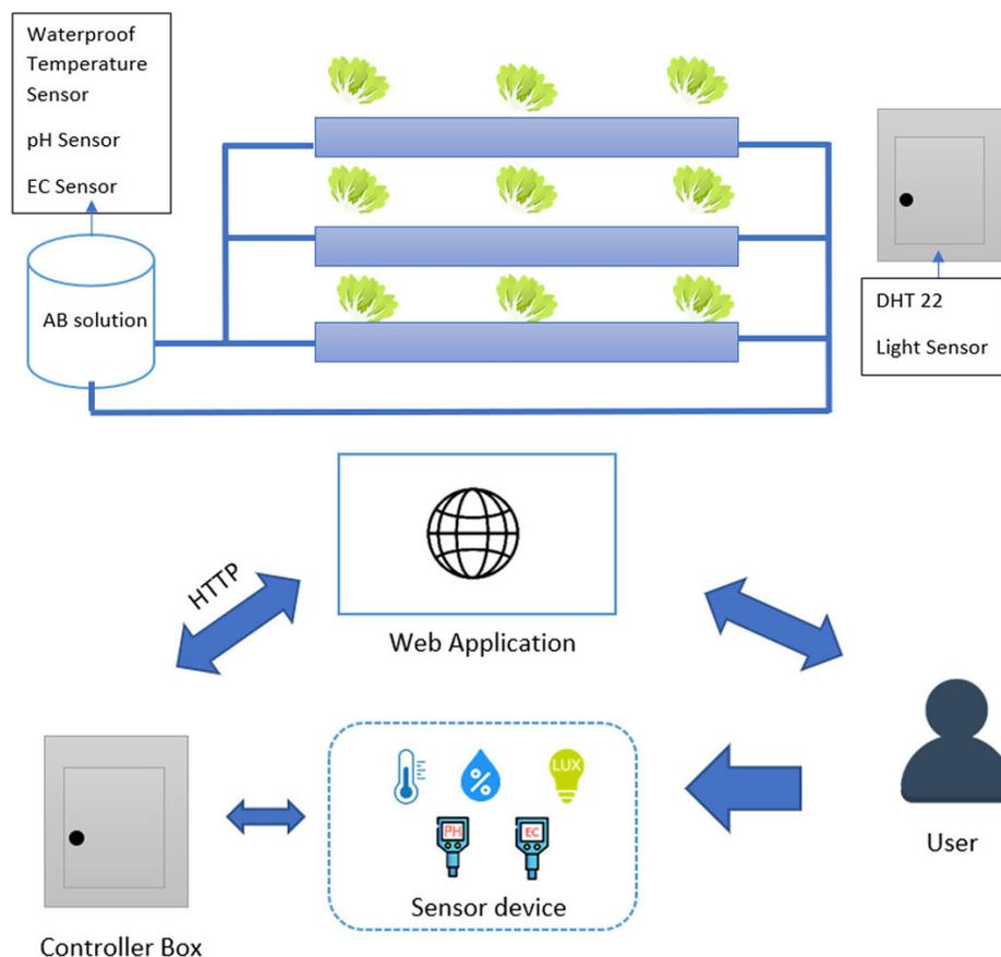
Fig. 2. Common sensors in hydroponics systems
