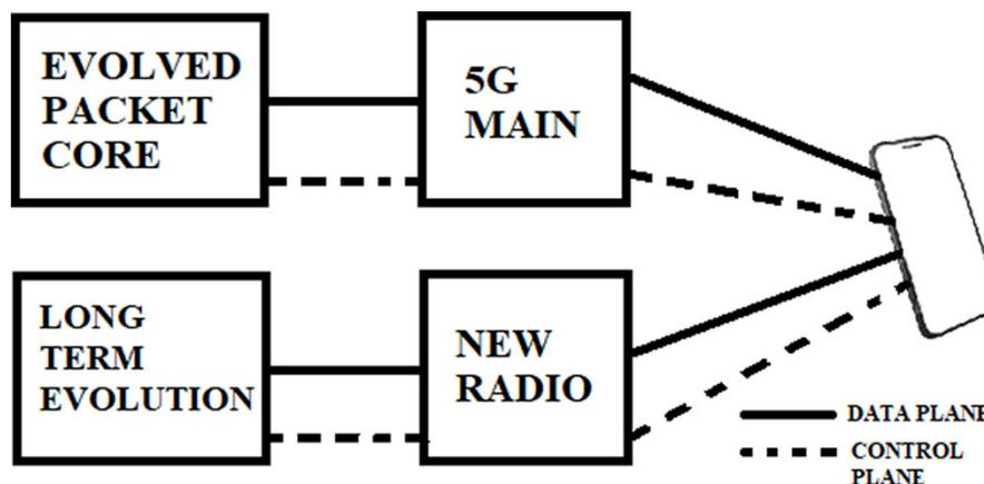
Fig. 2. Standalone architecture of 5G communication
