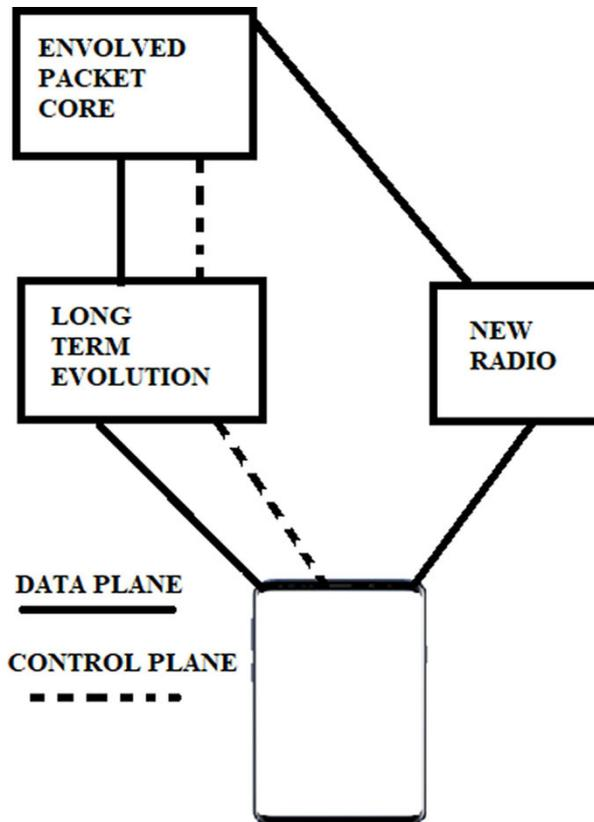
Fig. 3. Non-Standalone architecture of 5G communication
