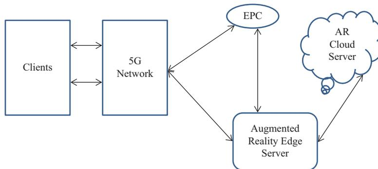
Fig. 2. Architecture of MAR with 5G & edge computing
