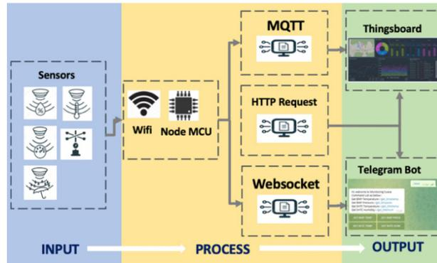
Fig. 2. Diagram of Data Retrieval Process
