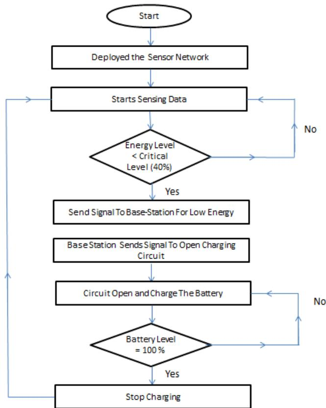
Fig. 4. The flowchart of the proposed work
