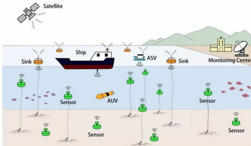
Fig. 1. A typical scenario of IoUT
