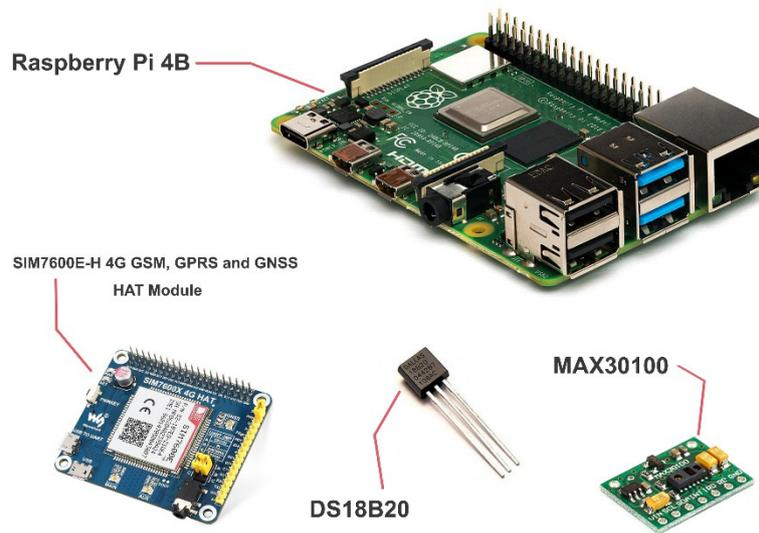
**Fig. 1.** Raspberry Pi 4B with SIM7600E-H 4G GSM, GPRS and GNSS HAT module, DS18B20 body temperature sensor and MAX30100 pulse oximeter
