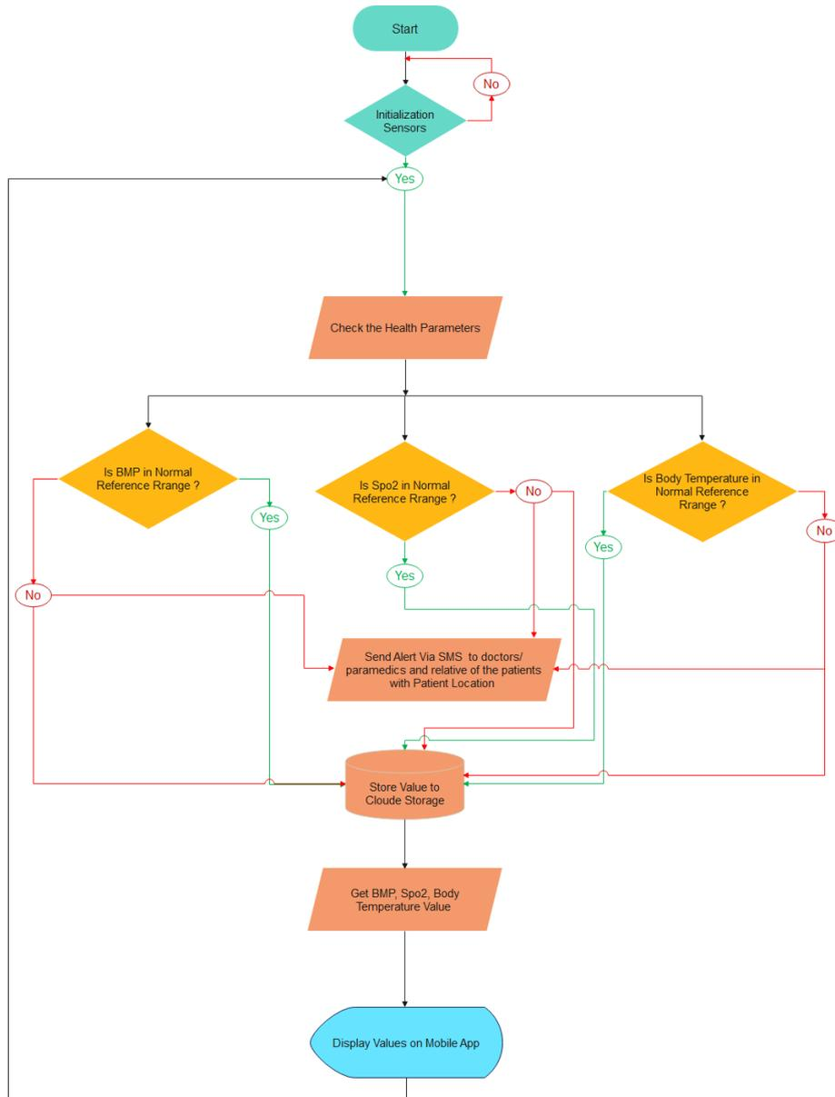
**Fig. 3.** IoT based smart healthcare monitoring system flow chart
