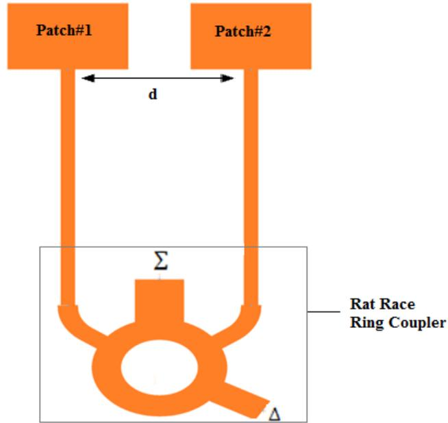
Fig. 2. Simulated design structure of the antenna array system
