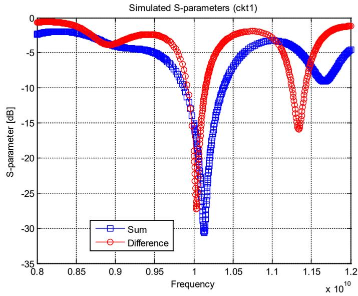
**Fig. 6.** Simulated S-parameters of  $\Delta$  and  $\Sigma$  ports
