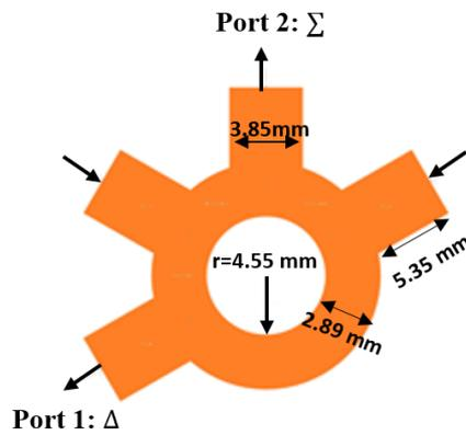
Fig. 4. The layout design of the simulated rat race coupler
