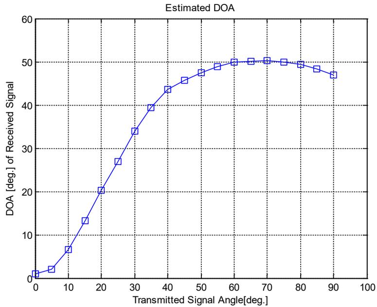
Fig. 8. The estimated AoA/DoA versus Transmitted signal (true) angle
