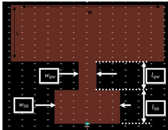
Fig. 3. The layout design of the simulated single patch antenna
