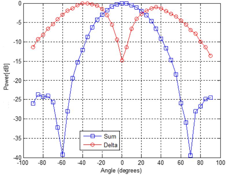
Fig. 7. Radiation patterns of  $\Delta$  and  $\Sigma$  ports
